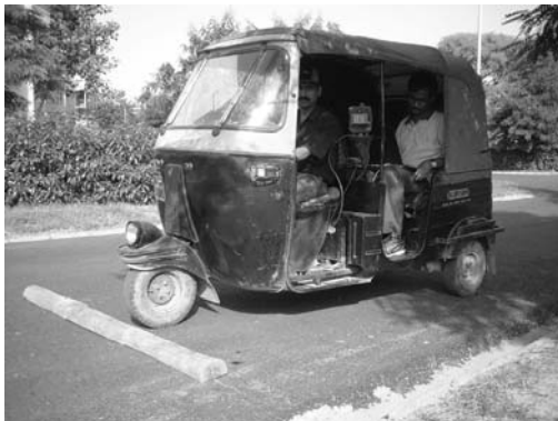
Fig. 1 Bajaj Auto rickshaw- rear engine 4 stroke, petrol model
