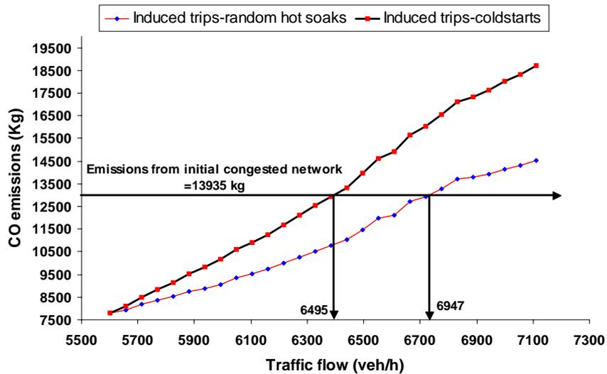
Figure 3: Identification of the break-even point for CO
